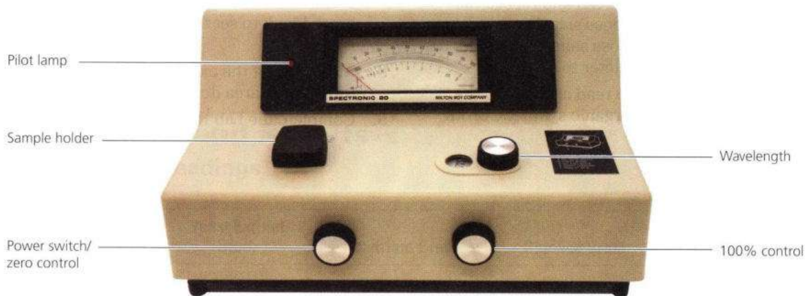
Figure 2 The Bausch & Lomb Spectronic 20 spectrophotometer
