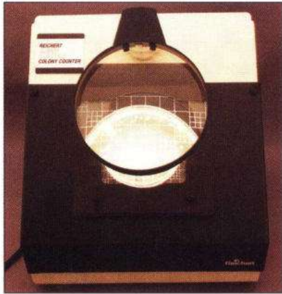
Figure 3 Quebec colony counter for the enumeration of bacterial colonies
