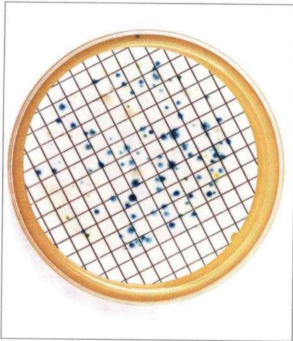
Figure 2 Development of colonies on a membrane filter following incubation
